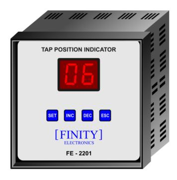
TPI's (Tap position indicator) purpose is to read, indicate, count and transmit the present tap which transformer is working on. From OLTC three output terminals are extended up to TPI named as Max, Com and Min.
